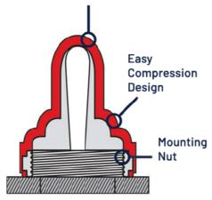
Switch boots are silicone-molded protective coverings that shield mechanical devices and electrical inputs from outdoor contaminants and environmental hazards, including, oxygen, water, saltwater, dirt, sand, bacteria, oil, and ice.
